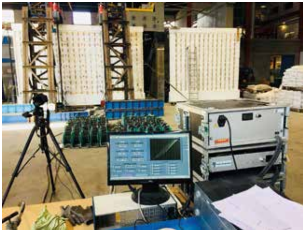
Experimental tests carried out at the Eucentre of Pavia to confirm the functioning of the ISOTEX construction system such as shear walls.
